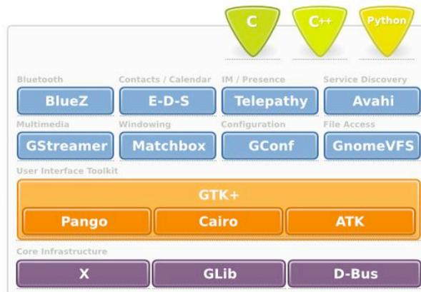
Figure B.2: GMAE software stack
